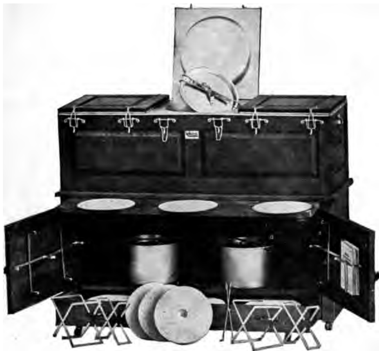
FIG. 77.—“Caloric” Fireless Cookstove, with storage cabinet below. The equipment consists essentially of three kettles with seamless aluminum lining , six radiators, trays, baking racks, radiator racks and tongs. The covers are equipped with valve that allows the excess steam to escape.
